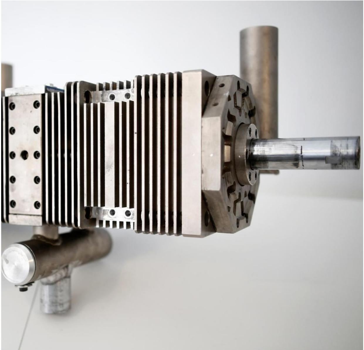
This is the prototype of the linear combustion engine. It generates electricity that can be used by an electric vehicle
